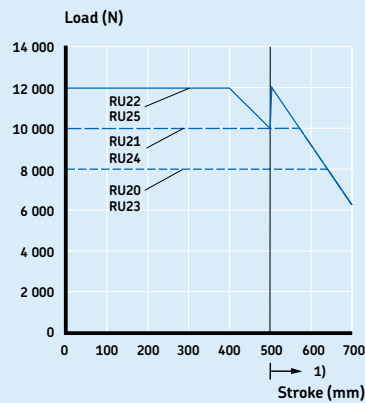
Push load limit, safety factor S=2 1) retracted length extension at stroke >500 mm
