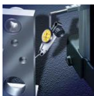
Perpendicularity using TESATAST
